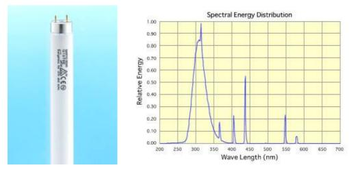
UV-B lamps emit ultraviolet rays between 280nm and 360nm (at peak 306nm). The spectral energy distribution suits to test the ultraviolet resistance of paints, plastics and rubbers. They are also used for the special light sources for inspection and analysis.
