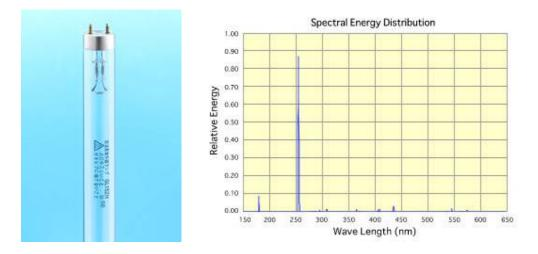
The ozone lamp(a short-wave germicidal lamp) made of quartz glass transmits UV rays at 185nm wave length that generates ozone, as well as germicidal UV rays at 253.7nm. The ozone lamp is best used for photomask and display cleaning, surface treating, air-disinfecting and deodorizing purposes.
