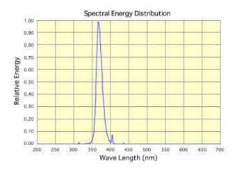
These lamps effciently emit near ultraviolet rays at 315nm- 400nm which have strong photochemical and fluorescent effects.
