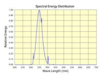
These lamps efficiently emit near ultraviolet rays at 315nm- 400nm which have strong photochemical and fluorescent effects.
