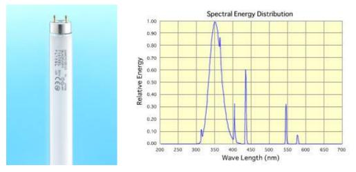
Like BLB lamps, these lamps emit a highly concentrated radiation between 315nm and 400nm (at peak 352nm). Other specifications are similar to those of general fluorescent lamps for illumination. They are used for trapping insects, luring lamps, photosensitization and photochemical reactions.
