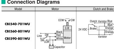
The direction of motor rotation is as viewed from the shaft end of the motor.
