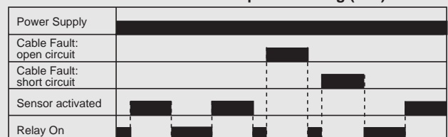
Namur sensor wired for Space Sensing (N/C)
