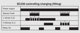
Note: F = Flashing LED to indicate sensor fault
