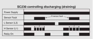
Note: F = Flashing LED to indicate sensor fault
