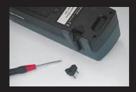
Apart from the standard aperture with a 3 mm diameter, we also offer easily exchangeable apertures with  $1.5 \times 1.5$  and  $2.5 \times 1$  mm which are particularly suitable for measuring
