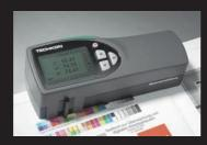
SpectroDens is particularly good at evaluating the Ugra/FOGRA-media wedge because the device toggles between colorimetric measurement without polarization filter and density measurement with filter at the push of a button.
