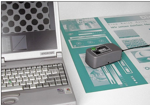
Digital MicroScope DMS 910 is positioned directly on the printing plate
